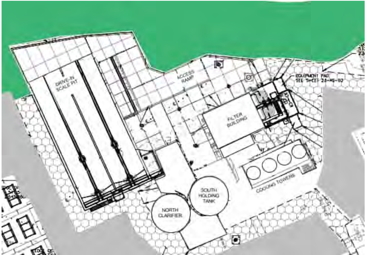
Figure #1 Proposed Rolling Mill CCW Site Plan Upon Project Completion Phase 2 Charter Steel Saukville Rolling Mill CCW Improvements
